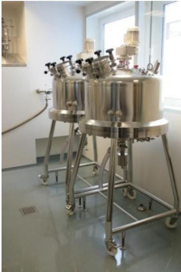
Resin conditioning vessels, self-draining Sanitary
