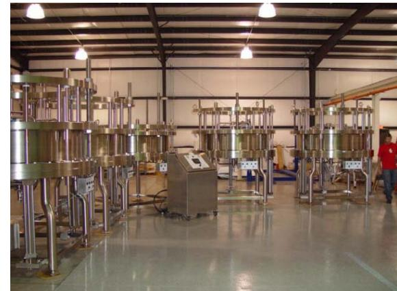
Proxcys Axial Biostream columns variable bed height 600 mm (Acrylic) and 1600 mm (Hastelloy). Hydraulic actuator.
